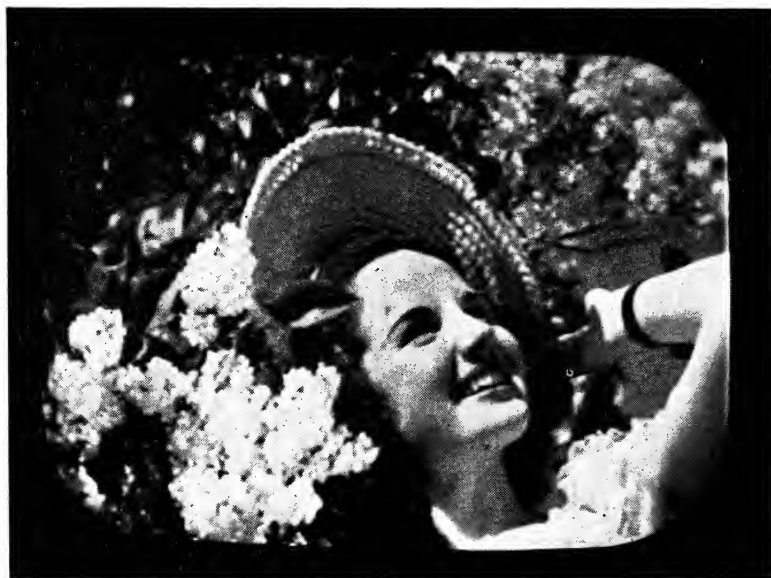
Fig. 7. Picture transmitted with 4.5-mc cutoff frequency, crispended.
